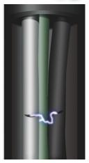
ogy to monitor the circuit for the presence of normal and dangerous arcing conditions. It will analyze ... an arcing event and determine if it is hazardous, in which case it will interrupt power to the line."
